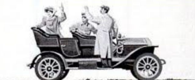
1907 KNOX WATERLESS was advertised as the "car that obviates the tow." The makers claimed that their air-cooled engine never overheated, thanks to hundreds of pins screwed into the cylinder walls to carry off engine heat.
